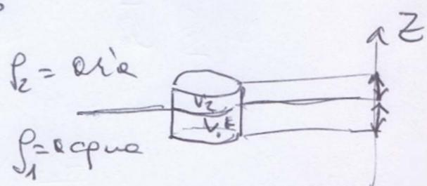
$$-\rho_c V_1 g + \rho_1 V_1 g + \rho_2 V_2 g = \phi \quad \text{equilibrio}$$
